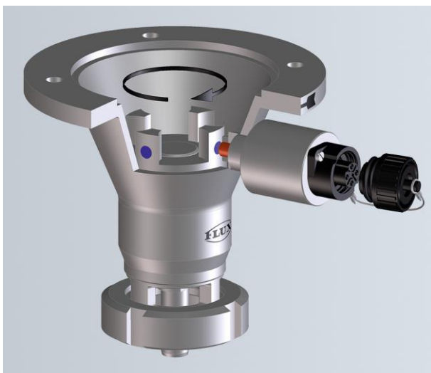
During rotation of the pump shaft four magnets switch the reed sensor in succession.
