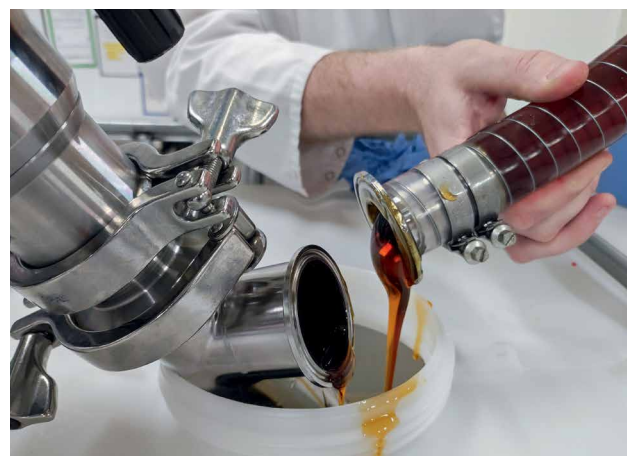
Pumping viscous golden syrup with the VISCOPOWER F 580 progressive cavity pump in a biscuit factory.
